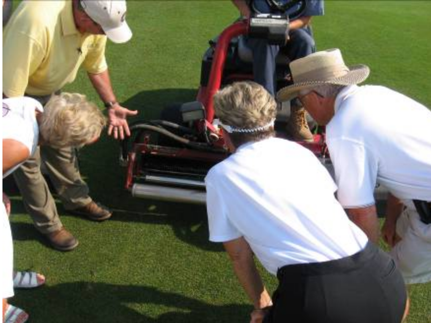
Superintendent Craig Foley describes how verti-cutting reels are different than normal mowing reels. These reels are vertical reels that thin out the turf grass.
