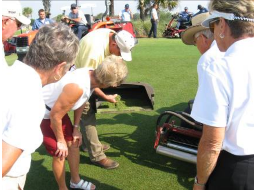
Craig shows how the grass is removed from the green using the verti-cutting mower
