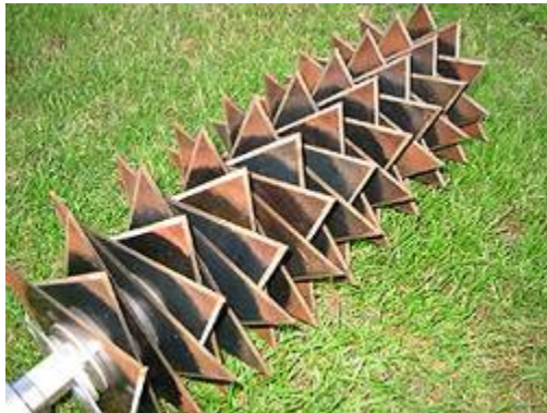
Superintendent Craig Foley describes how verti-cutting reels are different than normal mowing reels. These reels are vertical reels that thin out the turf grass.
